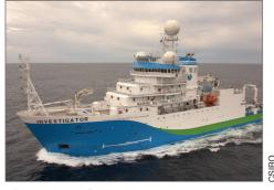
The Research Vessel *Investigator* is packed with scientific equipment that can map the sea floor at any depth. It can also reveal the composition of the sea bed 100m below the sea floor.
